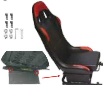
Attach the seat to the back frame by using four screws and nuts. For that, slide the seat backwards by pulling up on the handle underneath. Screw the seat to the brackets on the front end first. Then, slide the seat forward (again use the handle for this) to expose the holes on the back of the rails. Now attach the back to the brackets.
