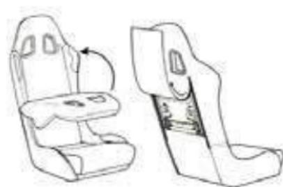
The seat is folded for easy transportation. To lock the back into place, open the flap at the rear of the seat, fold it upright and lock the 2 securing rods into place on the left and right edges.
